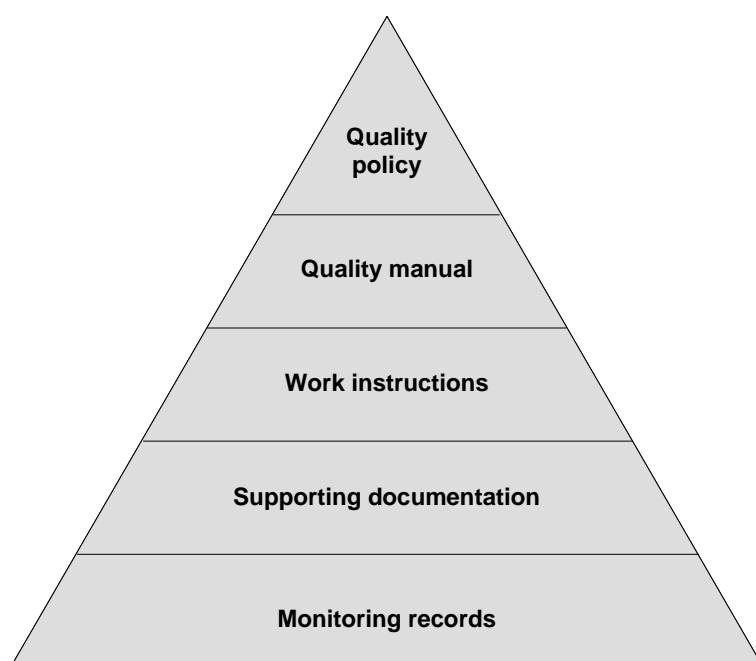
Figure 2.7: Basic structure for a quality management system
